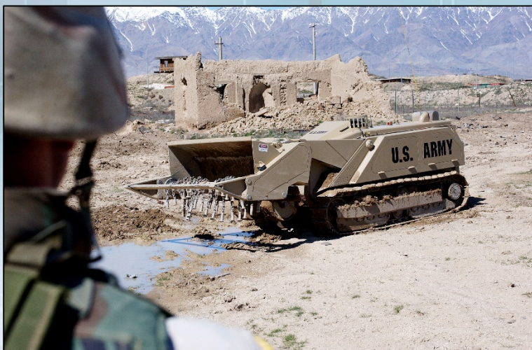
Army Staff Sgt. Bauer Ronald, of Company B, 367th Engineer Battalion, operates an MV-4 Flail. The MV-4 is a remote-controlled mine-clearing device. Photo by Spc. Jason Krawczyk, USA. (Retrieved from http://archive.defense.gov/news/newsarticle.aspx?id=31387 )
