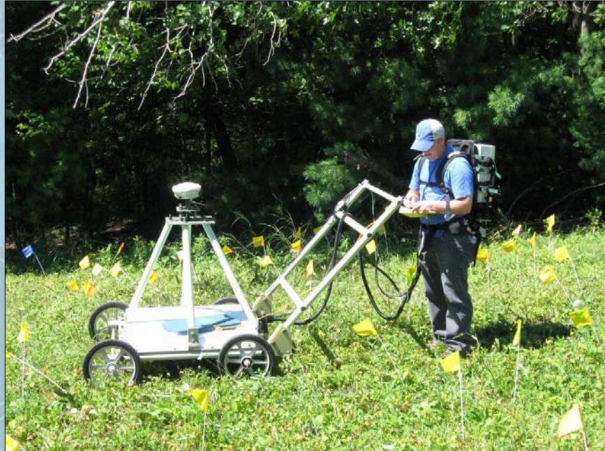
Andrew Louder, monitoring response geophysicist, uses a Time-Domain Electromagnetic Towed Array Detection System tool to map the subsurface at New Boston Air Force Station, N.H. Contractors are using the TEMTADS to differentiate between unexploded ordnance and cultural debris below the surface as part of a UXO clearance program at the station. Photo: Air Force Space Command, August 2013. http://www.afspc.af.mil/News/Article-Display/Article/731517/ground-piercing-radar-guides-new-boston-uxo-crews/
