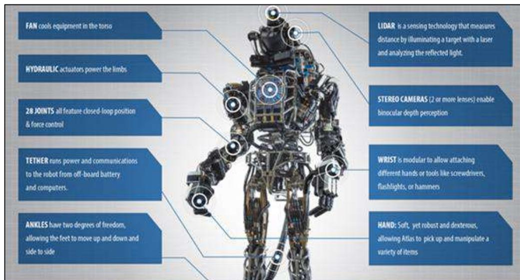
Figure 4. Overview of functions of the Atlas disaster response robot [15].
