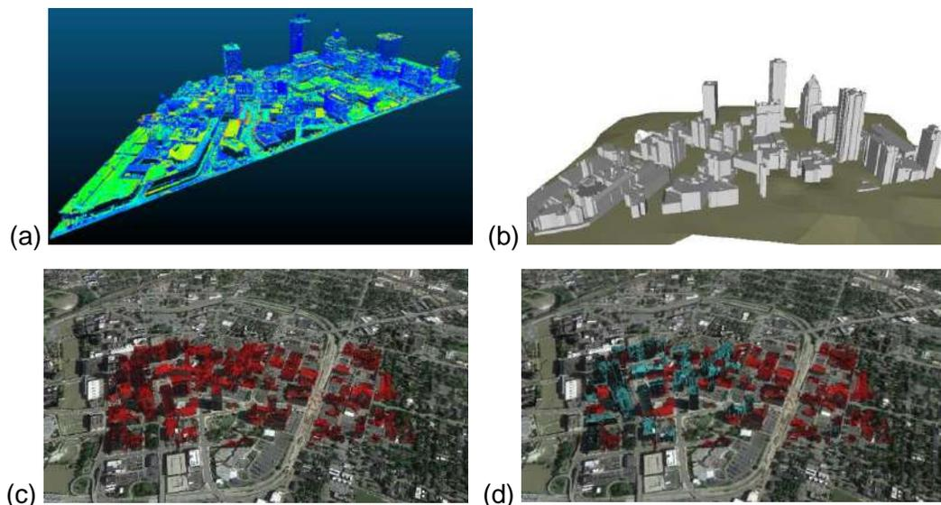
**Figure 1. Demonstration of image processing capabilities to extract individual building characteristics from point cloud data such as LiDAR: (a) data points from aerial LiDAR survey of downtown Rochester, NY, (b) resulting watertight building models, (c) rendering in Google Earth, and (d) ability to select individual buildings based on their geometric characteristics such as elevation. (Courtesy A. Lang)**
