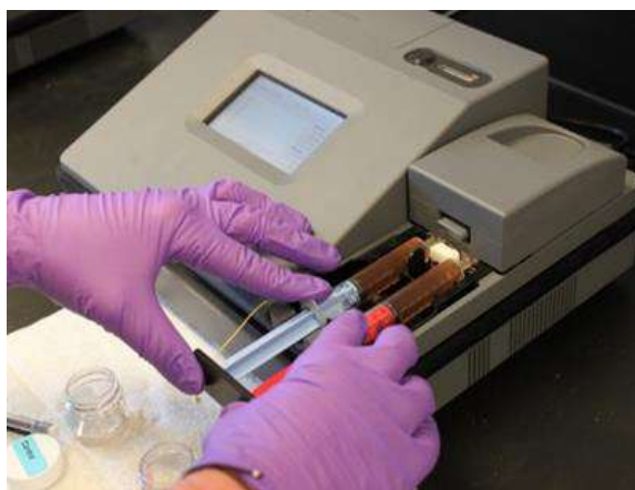
Figure 5. Simultaneous injection of control water (blue syringe) and test water sample (red syringe) for initiation of the ECIS test
