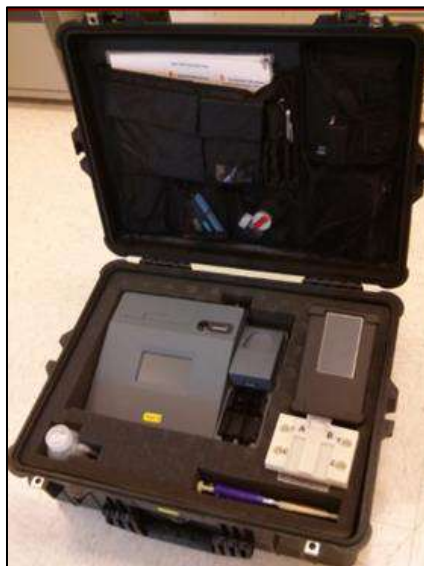
Figure 1. ECIS (instrument on the left) and ACE™ (instrument on the right) sensors with reusable supplies packaged in the ESB carrying case.
