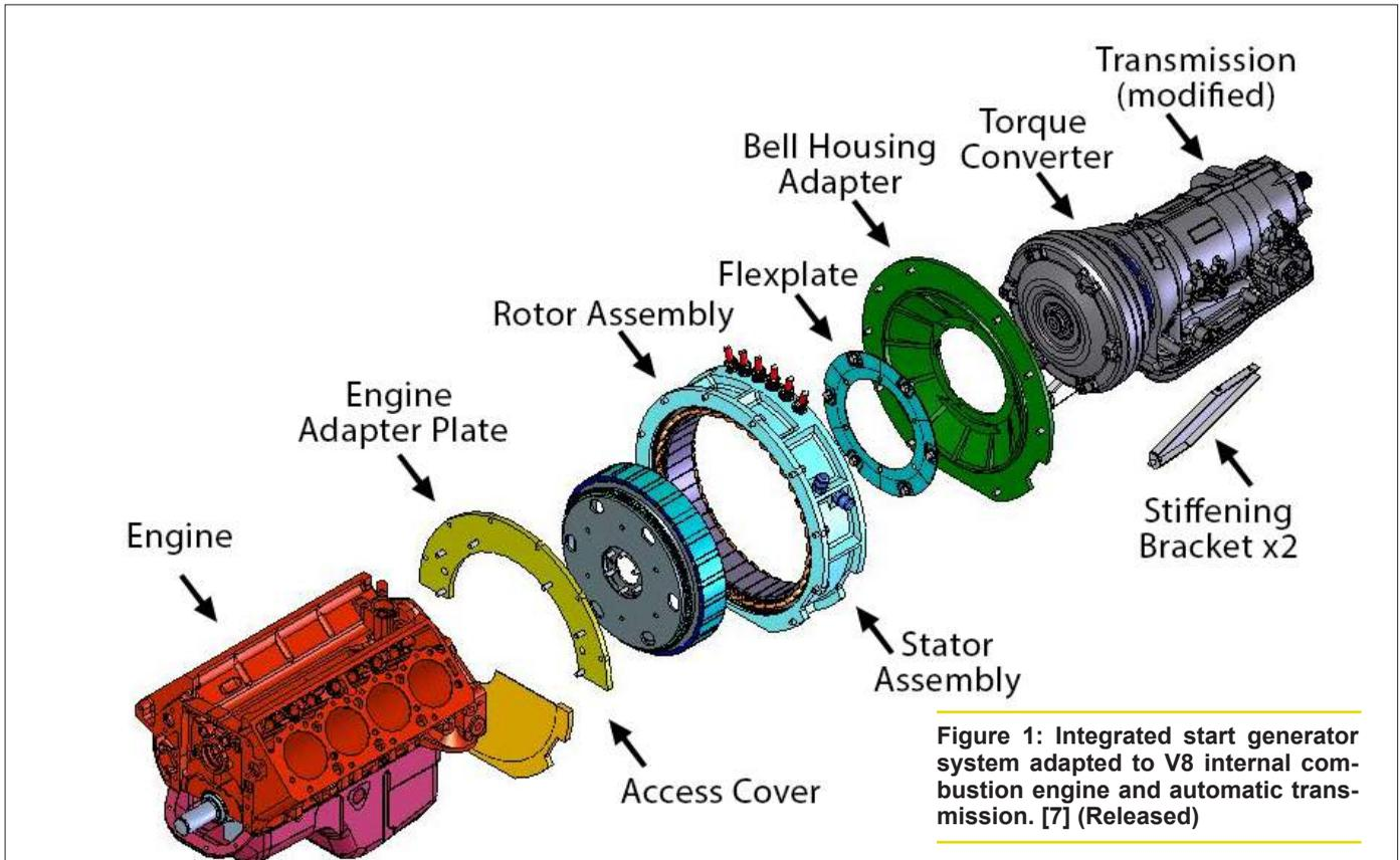
Figure 1: Integrated start generator system adapted to V8 internal combustion engine and automatic transmission. [7] (Released)
