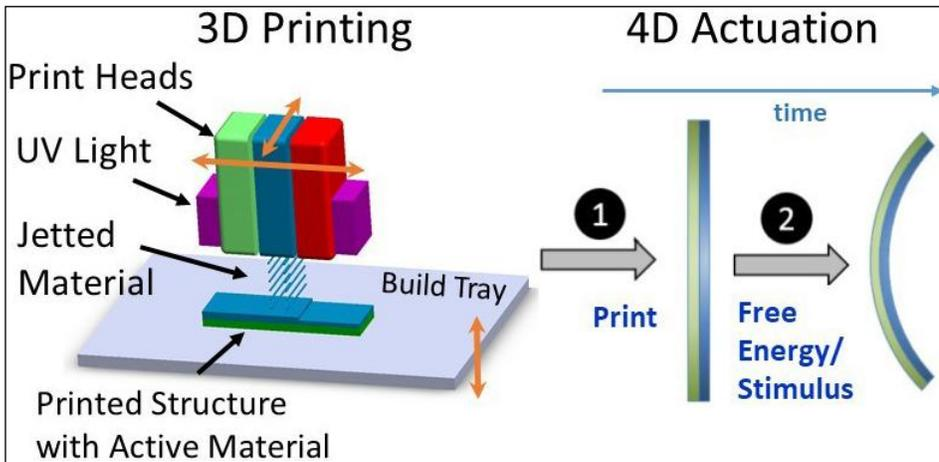
**Figure 1: Illustration of actuation of a 4-D printed object upon stimulus after a standard (polyjet) 3-D printing process. Adapted from [10].**
