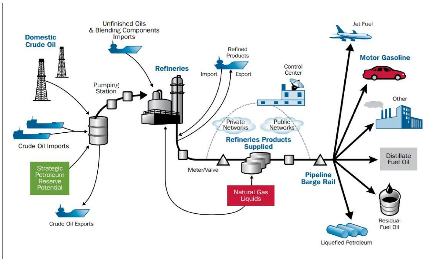
**Figure 4: Overview of the petroleum exploration, production, refinement, and distribution networks. Note how refineries are the linchpin—for the supply of liquid fuels [74].**
