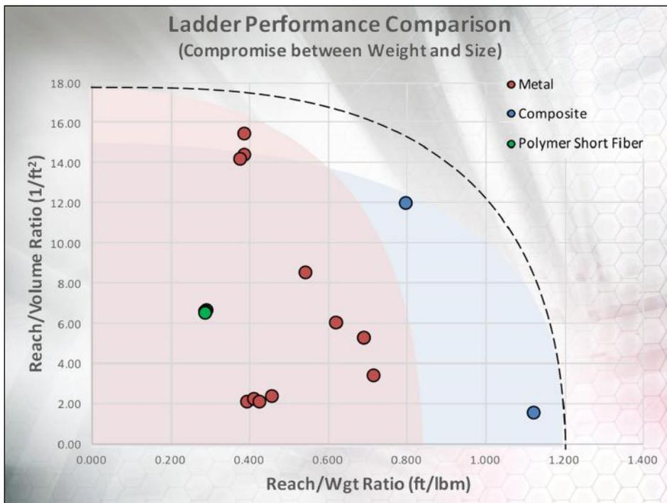
**Figure 1: State-of-the-art ladders present a compromise between low weight and small collapsed size. Carbon composites push the frontier toward lower weight but are not as compact when stowed as the best metal designs.**
