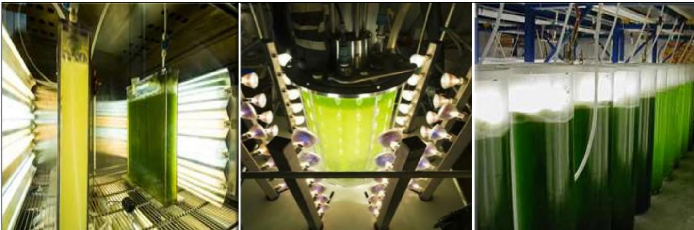
**Figure 4: Closed systems. Pictures showing different types of commercially available photobioreactor systems: bags, tubular, vessels etc. (Image courtesy of Robert Henrikson)**
