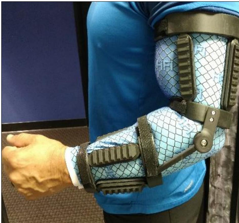
Figure 2: The full arm interface of the MOFO™ exoskeleton.
