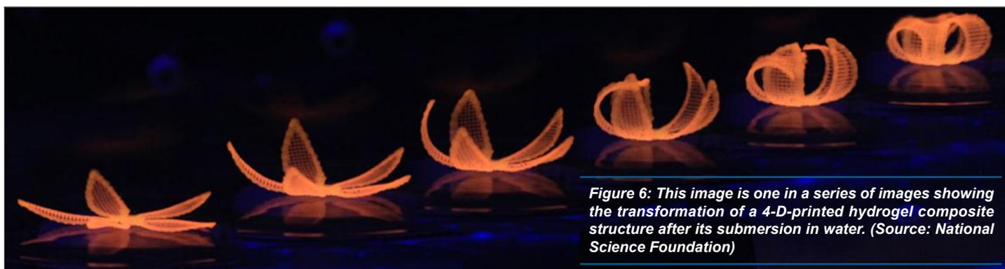
**Figure 6:** This image is one in a series of images showing the transformation of a 4-D-printed hydrogel composite structure after its submersion in water. (Source: National Science Foundation)
