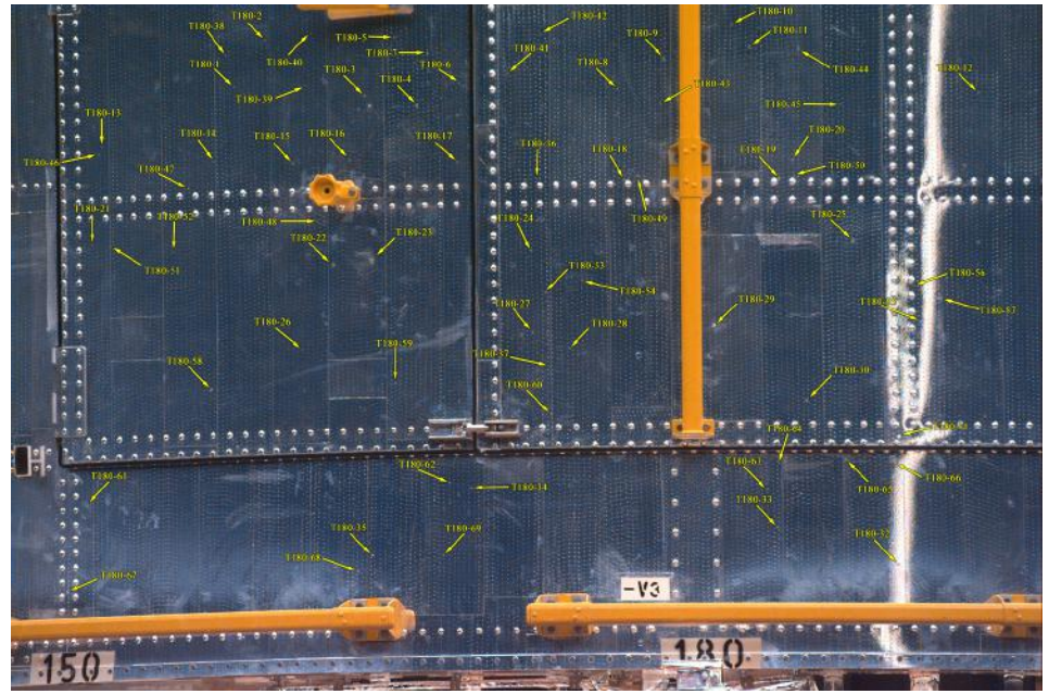
Figure 5. After in space repairs to the Hubble Space Telescope, the returned parts show many orbital debris impacts [26].
