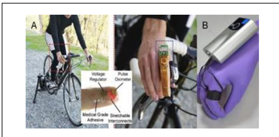
Figure 3. (A) Skin-mounted wireless circuit for pulse oximetry [16]. (B) Flexible glove biosensor with a portable potentiostat mounted to the back of the hand [17].
