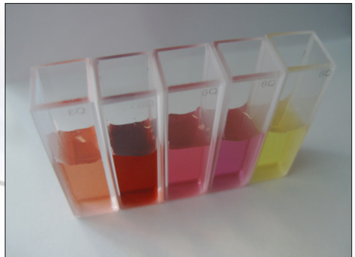
Figure 1. From right to left: Silver nanoparticles along with gold nanoparticles of decreasing particle size. (Released)
