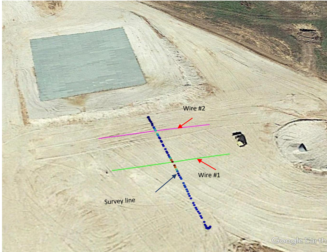
Overhead view of a test site for two subsurface wires
