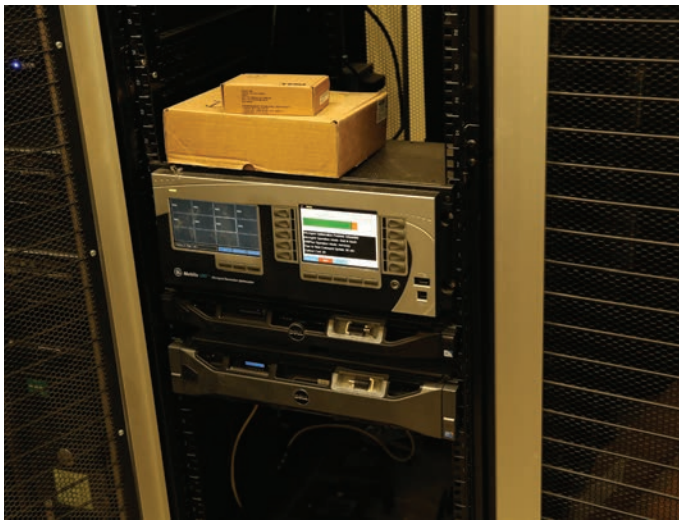
Figure 5-1. A General Electric (GE) U90 Plus Microgrid Generation Optimizer Monitors and Forecasts Solar PV Production at the USMC Air Ground Combat Center, Twentynine Palms, 2014 (Source: Mudd [209]).
