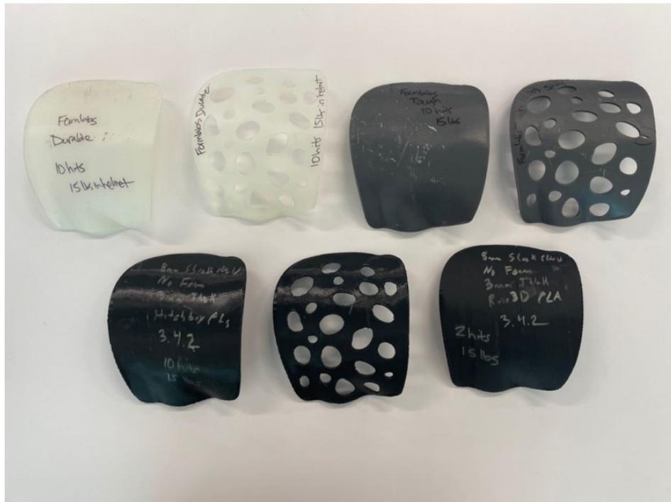
Figure #. Testing Guards (Top Row L-R: Formlabs® Durable resin, solid; Formlabs® Durable resin, holed; Formlabs® Tough resin, solid; Formlabs® Tough resin, holed; Bottom Row L-R: Hatchbox® PLA, solid; Hatchbox® PLA, holed; Raise3D® PLA, solid)
