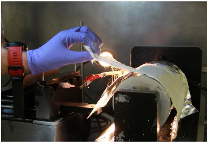
Figure 3-2. A Scientist From DEVCOM CBC Separates MOF Material From an Aluminum Surface After Electrospinning It (Source: DTRA [81]).
