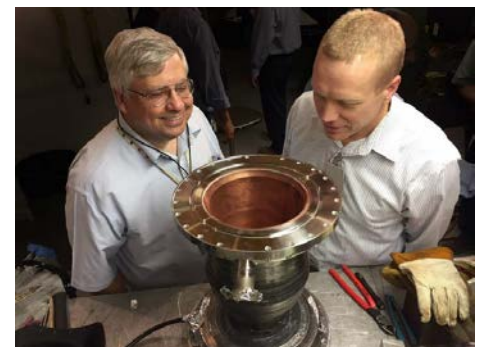
Figure 2. NASA Materials Engineers Dave Ellis and Chris Protz Inspect the First Additive-Manufactured GRCop Combustion Chamber (Source: Kilkenney [11]).
