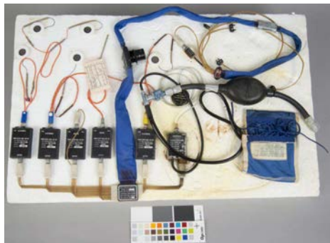
Figure 1. Wearable Biosensor Kit Used in the Apollo Space Missions to Track Astronaut Vitals (Source: National Air and Space Museum [1] ).
